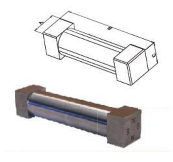
This applicator has the advantage of combining ease of use with 4 gap sizes in one unit. For best results it should only be used on solid substrates which are smooth. By simple rotating the applicator through  $90^{\circ}$  the next gap is placed onto the test surface.
